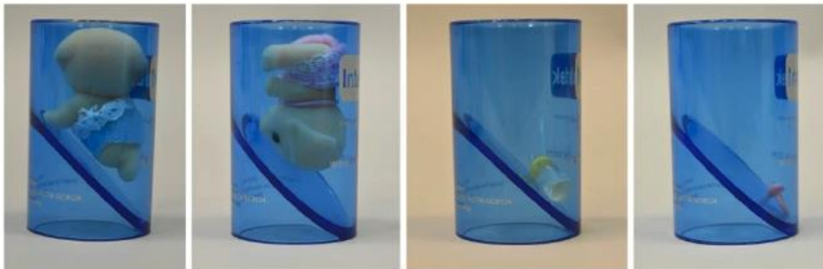
Figure 9 : Pictures of Calico Critters Yellow Labrador Twins toy and its accessories within the small parts cylinder. 18
