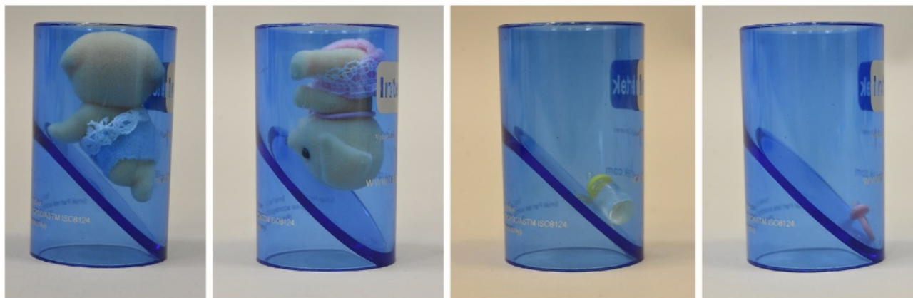
Figure 2: Exemplar parts fit entirely in Small Parts Test Cylinder
