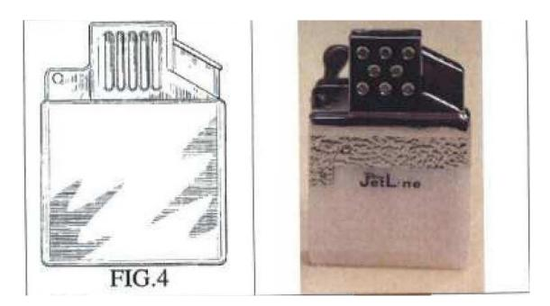
First, the windguard of the '274 Patent (Figure 4 on the left) has five vertical lines while defendants' ZTorch insert (on the right) is ornamented with a pattern of eight dimples, arranged in three horizontal, vertically offset rows. Second, defendants' Ztorch insert has a textured,
