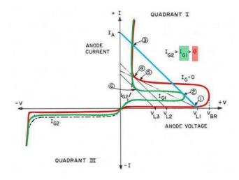
Id. ¶ 49 (citing Gen. Elec., SCR Manual fig.4.1 (D.R. Grafham & F.B. Golden, eds., 6th ed. 1982)). Though somewhat more complicated, the current-voltage characteristics of an SCR can be compared to those of the negative resistance device described in the patent. See '645 Patent fig.3 (graphing the I-V characteristics of a negative resistance device).
