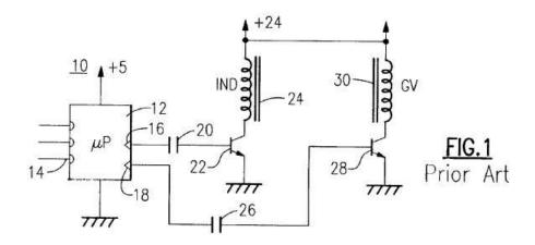
'645 Patent fig.1. As shown, the microprocessor has two outputs (labeled 16 and 18) used to trigger two different devices, which are activated using two actuator coils (labeled 24 and 30).
