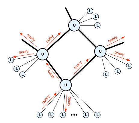
A LimeWire client (the leaf node "L" in the bottom-left of this figure) issues a query into the Gnutella network.
