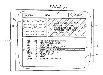
The specification explains that "[t]he viewer can move a cursor **48** vertically to highlight *one of the program listings* displayed in area **46**." ('864 patent col 5 ll. 19–20.) In Figure 2, the so-called program listings do not include scheduling information. Comcast's proposed construction
