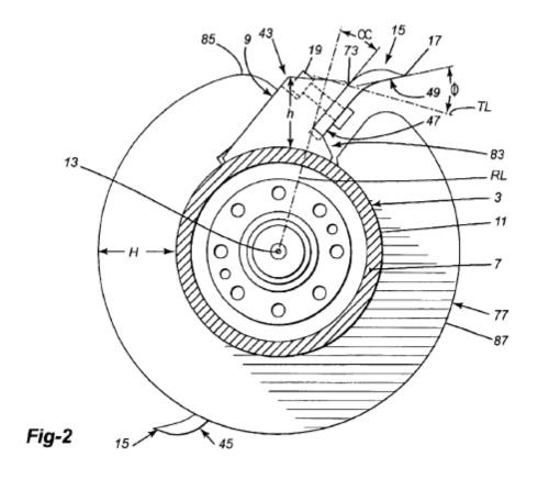
(Doc. 27-2 at 3). In this figure, "H" refers to the height of the protective guard/collar and "h" refers to the height of the block. The specification goes on to describe the height of "H" and "h": "Each collar 77 has a height 'H' equal to, or slightly greater than, the height 'h' of the block." (*Id.* at 5:56–57). Therefore, Cimaf emphasizes that the inventor has
