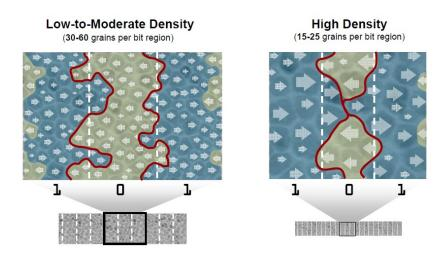
(Docket No. 771 at Ex. C at 24). So, as the density of the recording increases, the amount of noise or uncertainty in the signal also increases. (Docket No. 673 at 179). As seen below, the amount of noise is also affected by the specific sequence of bits written on the track.
