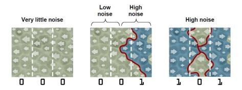
(Docket No. 771 at Ex. C at 25). This is correlated signal-dependent noise, because the noise signals from one boundary to the other move together, either attracting or moving away from each other. (Docket No. 673 at 179).
