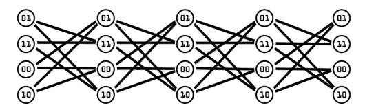
(*Id.* at 18). Through this trellis, one can trace a path that is equivalent to a specific sequence of symbols. (*Id.*). For example 100101, is shown below:
