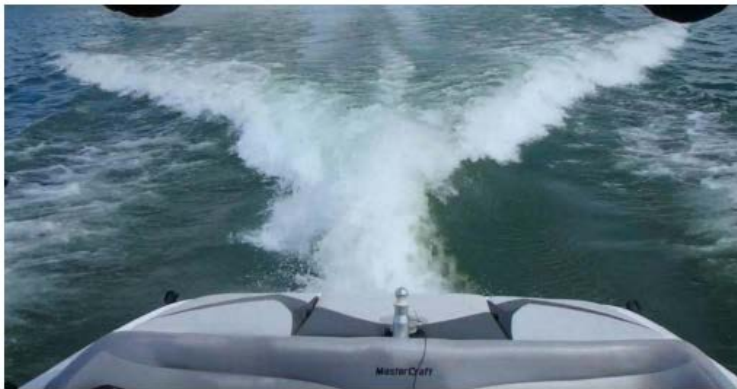
2010 MY MasterCraft X2, Port and Starboard Ballast Full, Starboard-side Surf Tab Deployed
