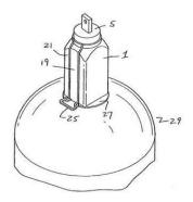
('587 Patent, Fig. 1 & Col. 1, ln. 63-65). In the illustration, the device (1) is shown surrounding the valve stem (5) of the cylinder (29). The tear strip (19) extends longitudinally along one side of the sleeve (21). (Id. Col. 3 ln. 4-7). Attached to the tear strip is a grip member (25) which "facilitate[s] tearing of the tear strip." (Id. Col. 3 ln. 26-27). At the bottom of the protective sleeve is a flange (27).
