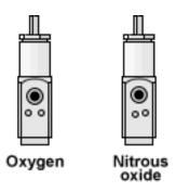
Given the slightly different location of the pin index holes, a user of oxygen cannot accidently attach his or her regulator to a cylinder containing nitrous oxide or some other sort of gas because the pin index holes will not line up with the prongs on the regulator.
