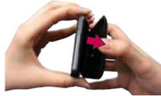
**1** Hold the phone with both hands, with the microphone facing upward. Then use the fingertip cutout to pull open the back cover (as shown above).
