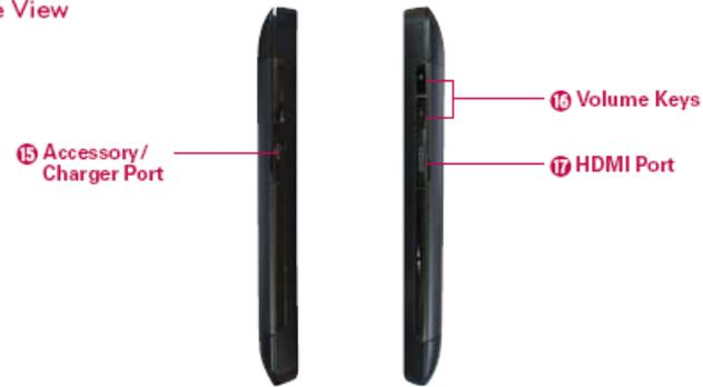
15. **Accessory/Charger Port** Allows you to connect the phone charger, USB cable, or other compatible accessories.
