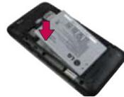
**2** Align the battery contacts with the terminals at the bottom of the battery compartment, then press the battery into place.
