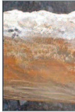
Figure 7 - Reactive fluid etching (left) and deposited scale (right).
