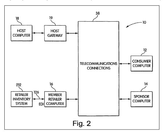
'830 Patent at Figure 2. Referring to Figure 2, the specification describes that "a consumer computer 12, a sponsor computer 14, and a retailer computer 16 are connected by a telecommunications connection 38 over the Internet to a host computer 18." *Id.* at 10:39–43.
