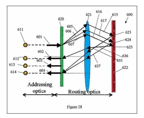
The specification describes that the switch uses a dispersion device 620 (shown in green), a focusing element 621 (shown in blue), and a Spatial Light Modulator ("SLM") 622 (shown in red), arranged in a folded architecture. '710 Patent at 43:41–43.
