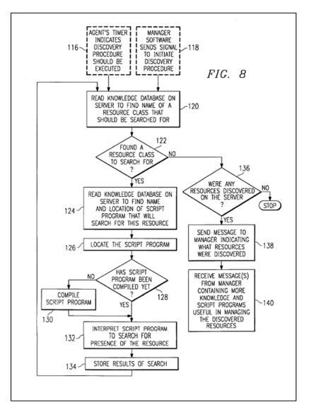
software systems for discovering resources on the network, monitoring aspects of resources, and taking recovery actions automatically in the event of an alarm condition.
