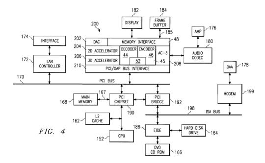
Defendants assert that the figure clearly shows that the Hard Disk Drive 164 is coupled to the EIDE 186 and the EIDE 186 is coupled to the ISA Bus 198. Defendants assert that an engineer might casually say that the Hard Disk Drive 164 is "coupled" to the ISA Bus 198, but would understand that the Hard Disk Drive is "connected to the EIDE 186 and through that to the ISA Bus 198." (Dkt. No. 60 at 17.) Defendants assert that, thus, "coupled" is not precise and not useful to one in the art.
