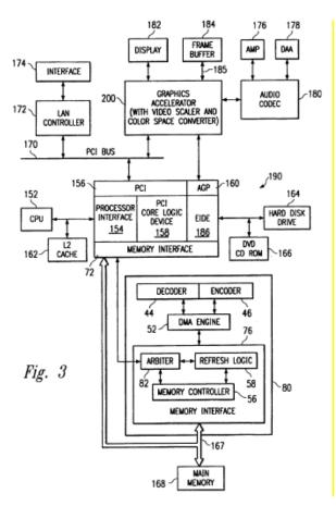
'194 Patent Figure 3. PUMA asserts that in Figure 3, the decoder/encoder 80 is connected to the graphics accelerator 200 and the display 182 through the core logic chipset 190. PUMA asserts that Defendants' construction would not encompass this embodiment due to the intervening core
