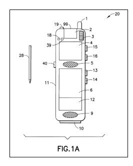
*Id.* at Figure 1A. The specification states that the device includes "a reading head 2, for example a camera or infra-red optical reading head (e.g. laser diode), suitable for capturing data and/or images . . . ." *Id.* at 5:38–40. The specification further states that "[t]he reading head is preferably interchangeable through the use of a clip-on enclosure 99, to allow the use of different types of reading heads." *Id.* at 5:42–44. The specification adds that "[a]n adjustment thumbwheel 3,
