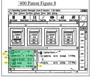
partitions of the secondary storage devices so that the user may add partitions to cabinets. That is, the "secondary storage partitions window" lists the secondary storage devices and their partitions. It should be noted, however, that while the partitions are *viewable* in the window, whether the partitions of a particular secondary storage device are actually displayed is a function of the state of the expander button (182).
