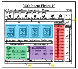
selecting the partition with the pointer and dragging the partition to the Active Selected Cabinet Visible Partition Window (90, in purple). Alternatively, the partition may be dragged to a cabinet listed in the Master Cabinet Visible Partition Window (91, in red). *Id.* at figs.1, 8–10, col.7 ll.1–33.
