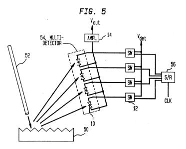
Chang '527 also discloses that "[e]ach switch 12 selectively applies a bias voltage supplied by a source of voltage  $V_{det}$  to the selected detector 10. All photo-detectors 10 supply their photocurrents to a single amplifier 14, which outputs an amplified signal  $V_{out}$ ." Chang '527 at
