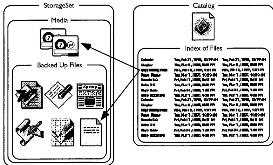
A StorageSet and its catalog. The catalog has pointers which locate the files on the media.
