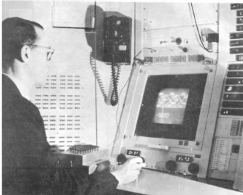
Figure 1.2: TX-2 OPERATING AREA — SKETCHPAD IN USE. On the display can be seen part of a bridge similar to that of Figure 9.6. The Author is holding the Light pen. The push buttons used to control specific drawing functions are on the box in front of the Author. Part of the bank of toggle switches can be seen behind the Author. The size and position of the part of the total picture seen on the display is obtained through the four black knobs just above the table. (Originally on page II.)
