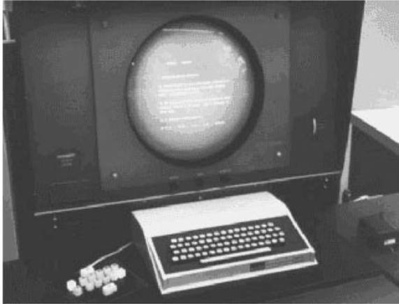
The oN-Line System display, keyboard and mouse
