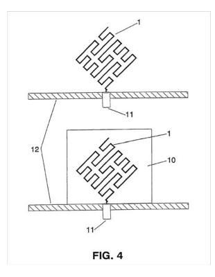
The loaded antenna patent claims antennae in which the radiating element consists of two different parts: a conducting surface and a loading structure. '762 at ABSTRACT. The conducting surface is described as consisting of a "polygon, space-filling or multilevel shape" and the loading structure consists of "a conducting strip or set of strips" connected to the conducting surface. *Id.* at 2:41-43.
