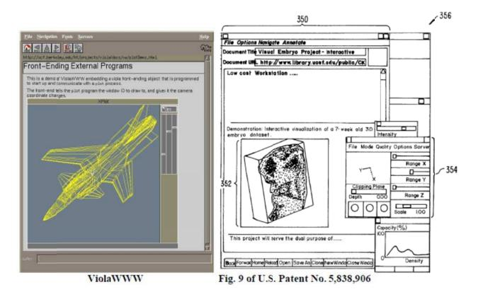
Both the ViolaWWW browser (on the left) and the preferred embodiment of the '906 patent (on the right) enabled a user to interact with a 3-dimensional image embedded in the middle of a webpage. In the ViolaWWW screenshot above, there are three slide controls to the right of the embedded image that move up and down; these rotate the embedded image on the X, Y, and Z axes. Similarly, in the preferred embodiment of the '906 patent shown above, box 354 has three
