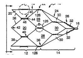
'025 Patent FIG. 1. Figure 1A further demonstrates that the filtering portion is centered along an axis running perpendicularly through the center of the circumference of the anchoring portion (i.e. concentrically aligned with).
