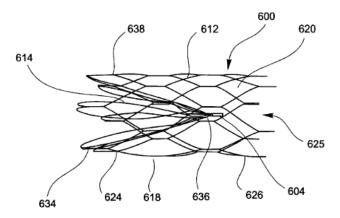
'025 Patent FIG 12A. This filter design, which is unique to the '025 Patent, is a "blood clot filter 600 further includ[ing a] filtering portion 614 which is concentrically aligned within lumen 625 of anchoring portion 612." '025 Patent col. 14:45-47; *see* Doc. No. 63 at 2.
