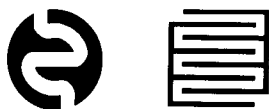
Fig. 13 Common pad patterns for conductive switches. (Courtesy of Shin-Etsu America, Inc, Union City, Calif.)
