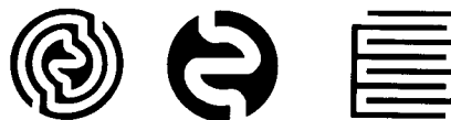
FIGURE 11.13 Common pad patterns for conductive rubber switches. (Courtesy of Shin-Etsu Polymer America, Inc, Union City, Calif.)
