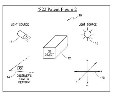
a computer screen. The 2D view of the 3D scene is from the observer's, or camera's (14), perspective and takes into account the light incident on the 3D object as viewed from the observer's perspective. The relative positions of the object, observer, and light sources are defined using a 3D coordinate system (20). '822 Patent col.1 ll.25–38, col.6 ll.28–57.
