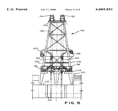
In this embodiment, the drill floor (114) is located above the base (110). Transocean contends that its construction results in defining the derrick (40) to include the base (110) that extends below the drill floor (114) and above the drilling deck (112).
