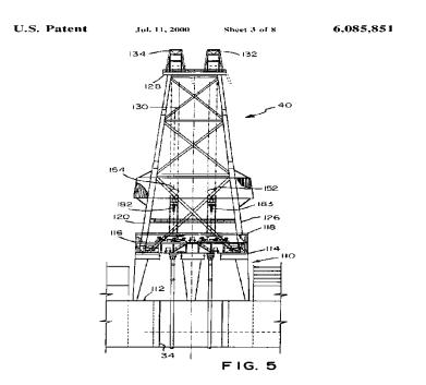
In this embodiment, the drill floor (114) is located above the base (110). Transocean contends that its construction results in defining the derrick (40) to include the base (110) that extends below the drill floor (114) and above the drilling deck (112).
