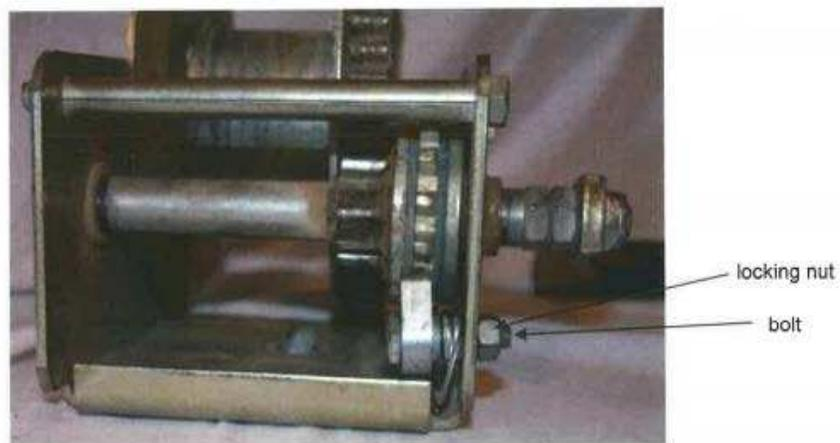
After the accident, various parts were recovered. The locking nut that attaches to the bolt from the outside wall of the winch was disconnected from the bolt. The bolt was disconnected from the winch, disconnecting the pawl—which was supposed to catch the ratchet gear and prevent it (and the attached handle) from spinning—from the ratchet gear. See Docket no. 52 at 3:
