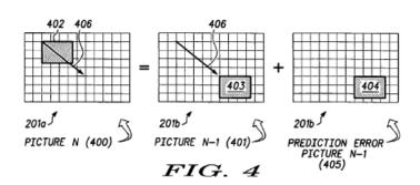
('374 Patent at Figure 4.) The Patents-in-Suit also disclose that the motion vectors themselves may be encoded by referencing other motion vectors. (*Id.* at 9:38-45.)
