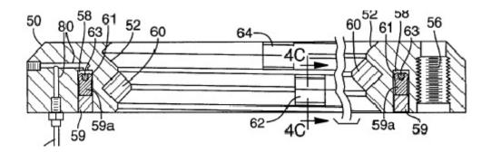
When hydraulic fluid is provided to the chamber above the seal portion, the seal portion expands under pressure. This expansion both seals the chamber and causes the piston to move downward and exert the forces that lock the bowl into place.
