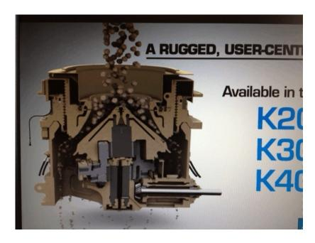
Because the operator of a rock crusher will want to make small rocks of different sizes (one inch, an inch-and-a-half, etc.) depending on the job, it is important to be able to adjust the spacing between the bowl and the cone. The spacing is usually adjusted by vertically moving the bowl closer to or farther away from the cone. Smaller rocks are produced by moving the bowl closer to the cone. Larger rocks are produced by moving the bowl farther away from the cone.
