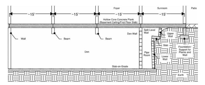
*Id.* at 4. The report notes that vibrations from the blasting created a horizontal crack in the lower wall:
