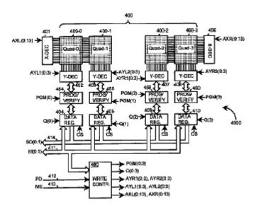
Dkt. #60-5, U.S. Pat. No. 5,890,192, Fig. 3. (Although each separate group of memory storage elements is labeled as a "quad" in Fig. 3, elsewhere the patent describes the group of storage elements as a "plurality of flash EEPROM cells 400 organized into four sub-arrays or quadrants, 400-0 to 400-3." <u>Id.</u>, col. 3, lns. 57-58.)
