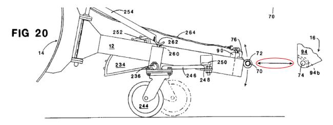
'690 pat., Figure 20 (emphasis added). There is no denying that the entire pipe -- as well as the entire plow assembly for that matter -- moves in a direction parallel to the longitudinal axis of the vehicle to connect the plow assembly to the vehicle as evidenced
