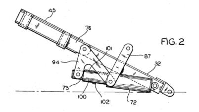
Through this assembly, extension of piston rod 73 pushes link 92 (made up of side members 94 and 95) forward, which causes the snowplow blade 40 and support 30 to tilt upward. ('624 patent, 5:47-51.)
