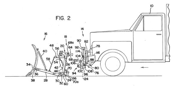
Specifically, the "frame assembly 20," when connected to "vehicle portion 14," extends in front of and above the vehicle's bumper. Additionally, the '329 patent discloses an actuator ("hydraulic cylinder device 42") connected to the support frame and an A-frame that, as described in the patent, pivots the A-frame about a pivot axis:
