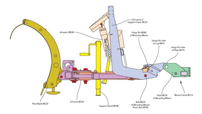
(Dkt. #126-4) (actuator labeled M646). Given the Federal Circuit's construction of "connected to" as encompassing both direct and indirect connections, it is also clear that the actuator is connected to the support frame (blue), and to the A-frame (pink) via the support frame, in order to accomplish the pivotal movement described in claim 45. Accordingly, Douglas is entitled to summary judgment of infringement on claim 47.
