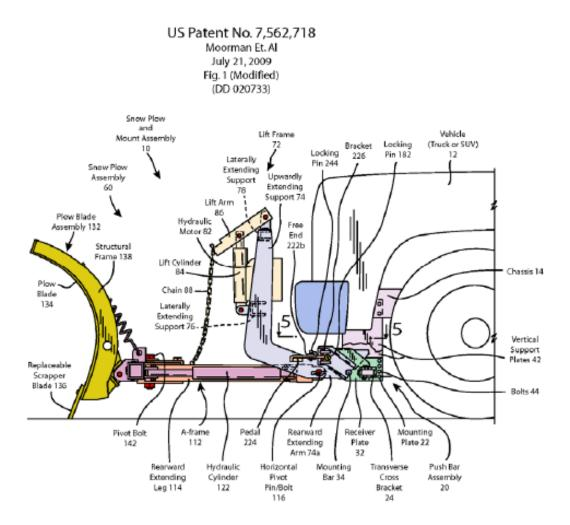
(Garris Report Vol. 3 (dkt. #128) ¶ 60.) The "upwardly extending support," labeled 74 in the modified figure, is an "extension in front of and above" the vehicle bumper. Buyers does not dispute that its products literally contain this element. (*See* Def.'s Resp. to PPFOF (dkt. #193) ¶ 154.)
