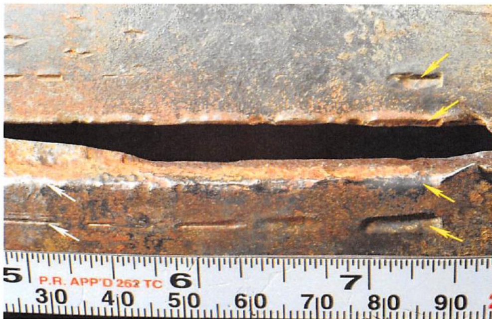
Figure 2 Close-up view of the split showing deep tong marks, indicated by yellow arrows, and shallow tong marks, indicated by white arrows.
