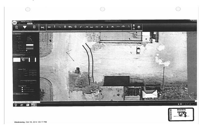
The diagram demonstrated Thompson's findings of two tire marks avoiding the adjacent roads and heading southbound through the parking lot with a definite turn in the marks' path. In addition, Thompson saw definite acceleration markings leading southbound to the body and no evidence of deceleration marks at any point on the path. Finally, Thompson noted clear evidence of steering input in the tire marks' pattern, signaling that the car was not "out of control."
