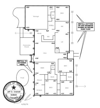
and area drain basins or repair sump pump" to repair the external drainage issues. The last page of the CCM Report included a sketch showing CCM's recommendations. The sketch shows suggested locations for the installation of sixteen piers around portions of the foundation and notes the
