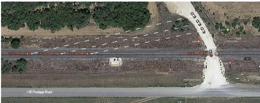
Figure 4 - Portion of scaled diagram showing impact and locations of locomotive and Ford at 4, 5, and 6 seconds prior to impact
