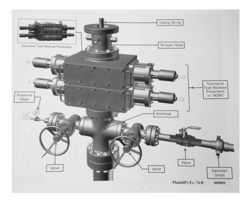
[¶7] Many months before the incident involving Horr, Merit had provided a "Washington" stripper head, along with the BOP, for the Basic crew to use when servicing Merit's wells. Significantly, the Washington head had a release valve that could be used to relieve pressure trapped between it and the blowout preventer. Without such a valve, the well would need to be "killed" to control the pressure.
